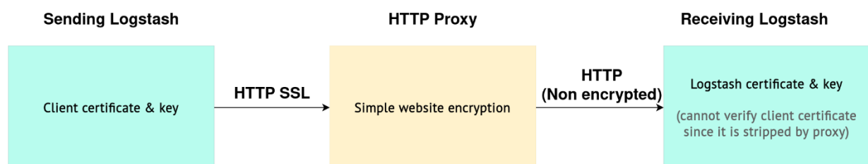
Figure 5: Logstash to Logstash communication through a HTTP proxy
