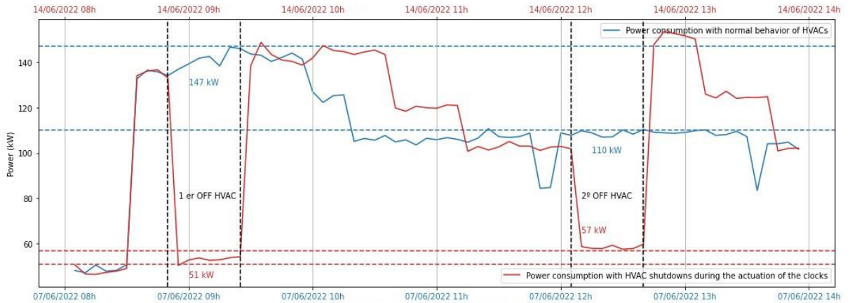
Figure 18 – Test of June 14 th / Psychology Faculty - Power consumption with HVAC shutdowns during the actuations with the clocks vs Power consumption with normal behaviour of HVAC
