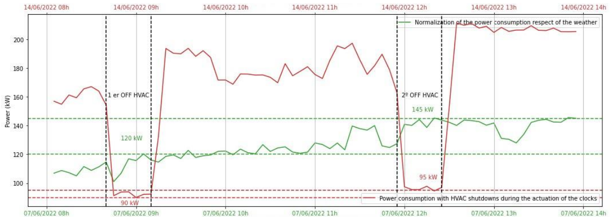
Figure 21 – Test of June 14 th / General Library and Documentation Faculty - Power consumption with HVAC shutdowns during the actuations with the clocks vs Normalized consumption power respect of the weather
